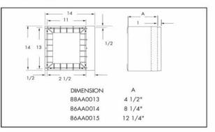
FIG. E- 86AA001- Duct Connector
